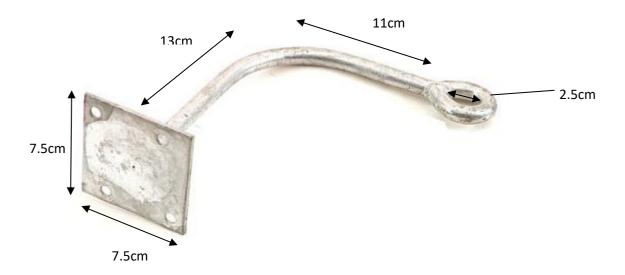
Similar to the Bracket 22, this bracket is used for fixing Clamps Dropwire on buildings and poles but has an extended arm to give additional clearance from guttering's & eaves.
